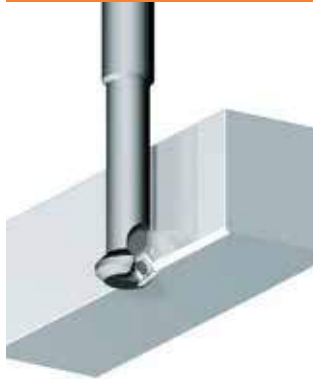
Rear surface Edge chamfering process
