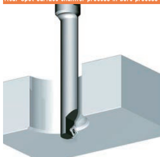
Rear Spot surface chamfer process in bore process
