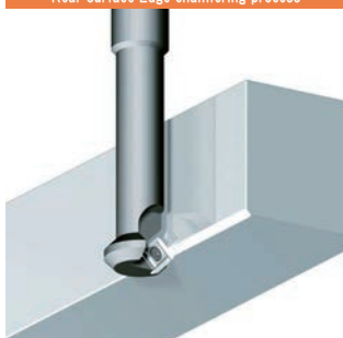
Rear surface Edge chamfering process
